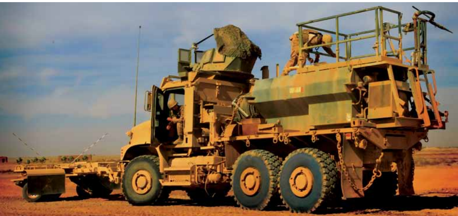
A construction vehicle belonging to the 9th Engineer Support Battalion, 2d Marine Logistics Group (Forward), sprays down a road during an operation in Helmand Province, Afghanistan, while building a main supply route in the Shir Ghazay area. (Photo by LCpl Katherine Solano, USMC)
