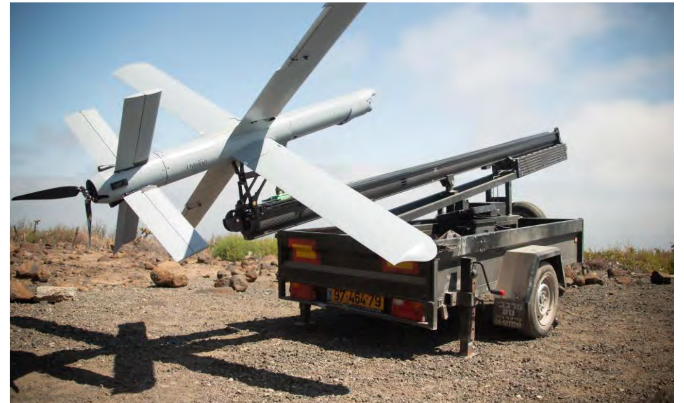
A Marine Corps Hero-400 loitering munition drone is staged before flight May 25, 2022, at San Clemente Island, California. (Photo by Marine Corps Lance Cpl. Daniel Childs)
