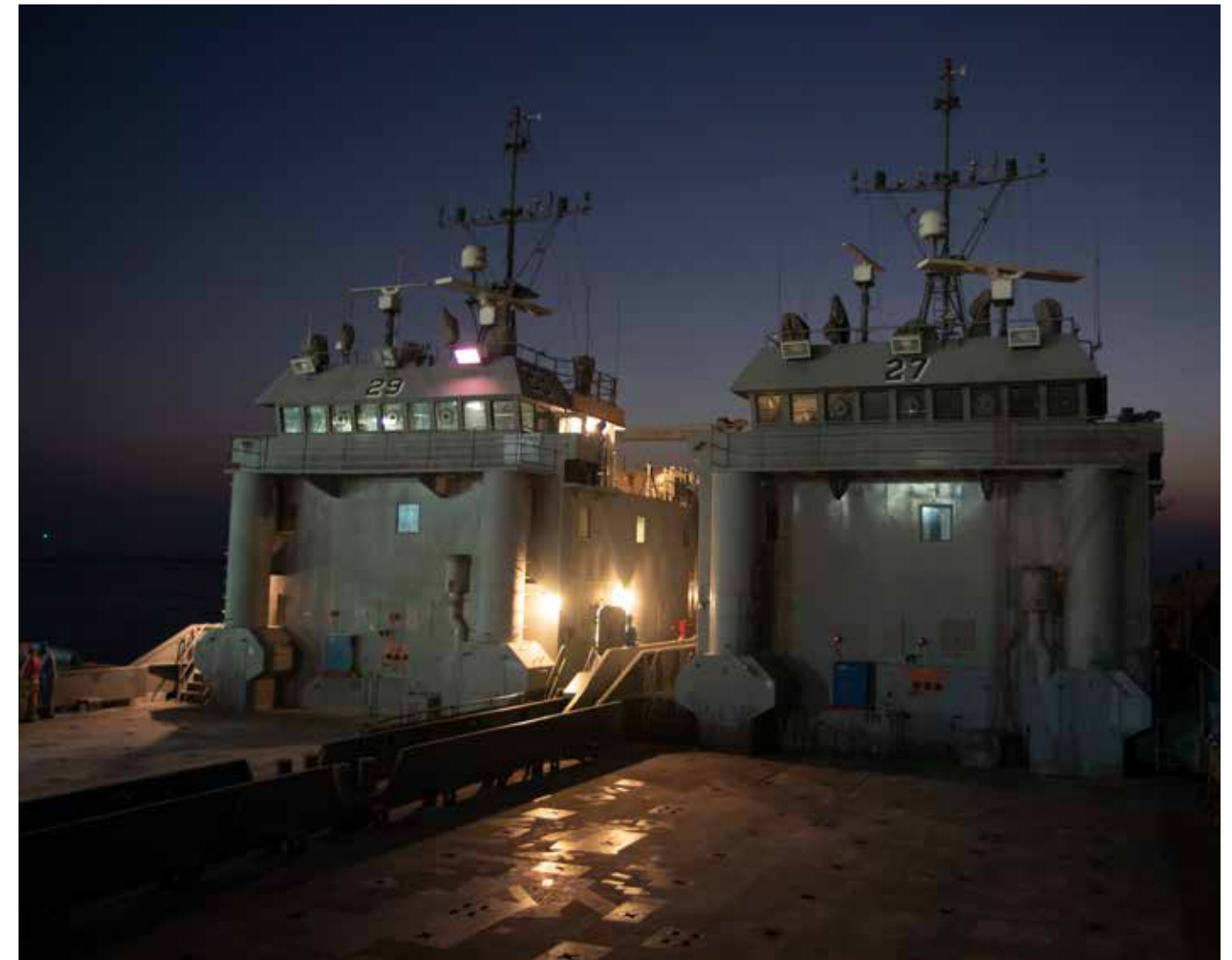
Two Army Landing Craft Utilities (LCU) are staged at the Kuwaiti Naval Base, Kuwait, before transporting to their new area of operations on Oct. 7, 2020. LCUs are capable of transporting wheeled or tracked vehicles and personnel from battle ships to land. (Photo by Staff Sgt. Christopher Osburn)
