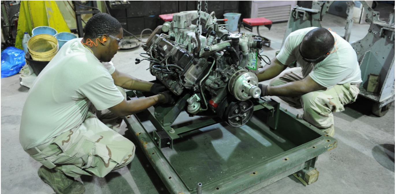
Anniston Army Depot heavy mobile equipment mechanics prepare a 6.5 engine at the TACOM Life Cycle Management Command Forward Repair Activity in Kuwait. (US Army photo)
