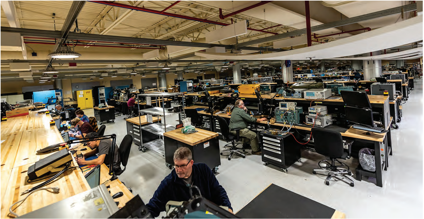
Tobyhanna Army Depot's electronic maintenance enclosure was designed in line with current trends and industry best practices. The 30,000-square-foot enclosure includes a raised floor that can easily be reconfigured for changing mission needs. It is certified according to aerospace quality standards and electrostatic discharge requirements. (Photo by Thomas Robbins)
