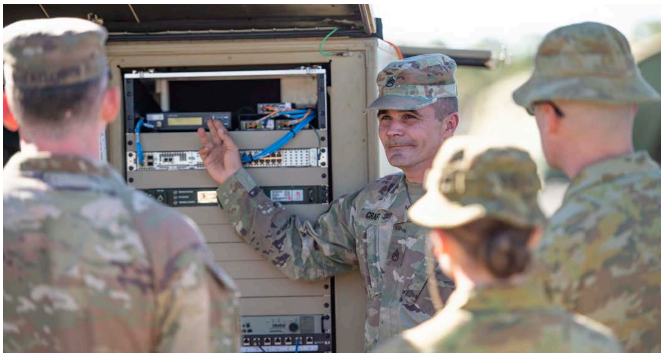
U.S. Army Staff Sgt. James Craft, signal support specialist, 10th Support Group, instructs American and Australian service members on how to operate a Satellite Transportable Terminal (STT). The STT provides seamless connectivity to strategic facilities for distribution of services throughout the tactical network. (Photo by Mass Communication Specialist 3rd Class Daniel L. Zink)
