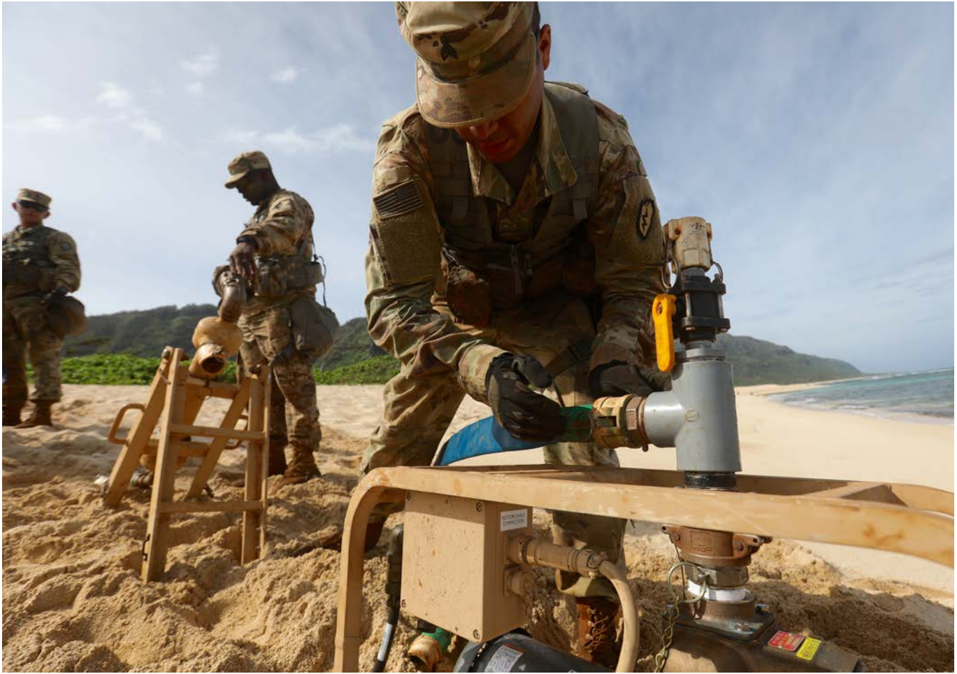
Soldiers from the 209th Aviation Support Battalion, 25th Combat Aviation Brigade, assemble a water pump while training on the tactical water purification system on Feb. 27, 2018, near Dillingham Airfield, Hawaii. (Photo by Sgt. Ian Ives)
