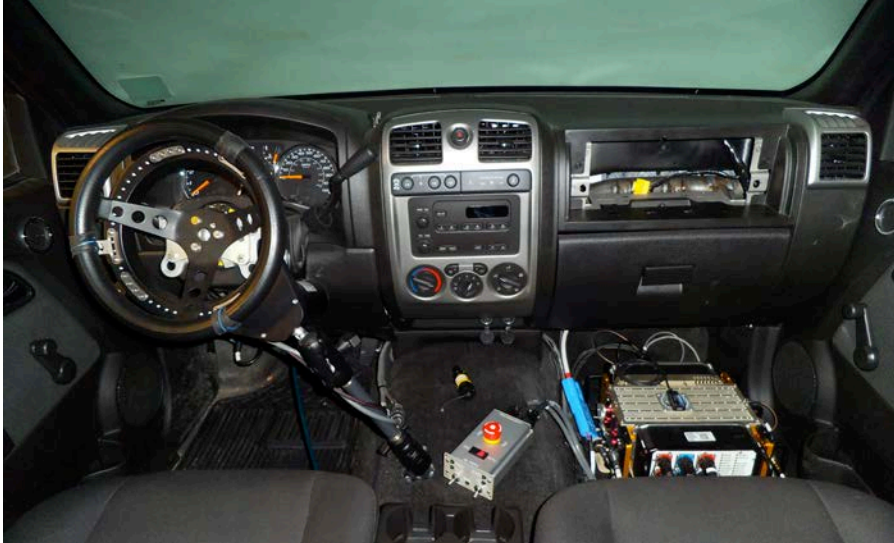
This Pronto4 robotic applique kit, installed on a Chevy Colorado, was successfully tested and is currently in use for target training. (Photo courtesy of Kairos Autonomi)
