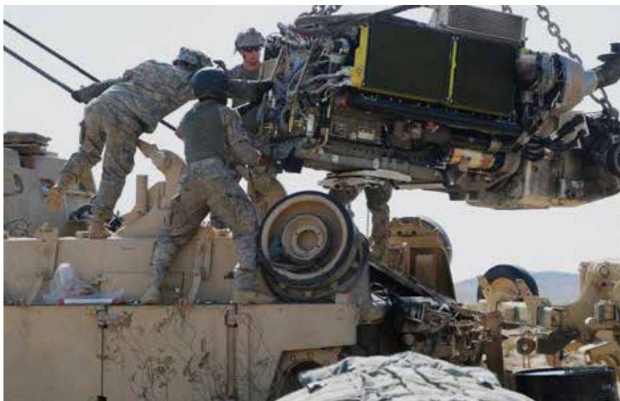
Crew members and mechanics from G Forward Support Company, 101st Brigade Support Battalion, 1st Armored Brigade Combat Team, 1st Infantry Division, reinstall an engine during National Training Center Rotation 16-08 in August 2016. (Photo by Capt. Jonathan Camire)
