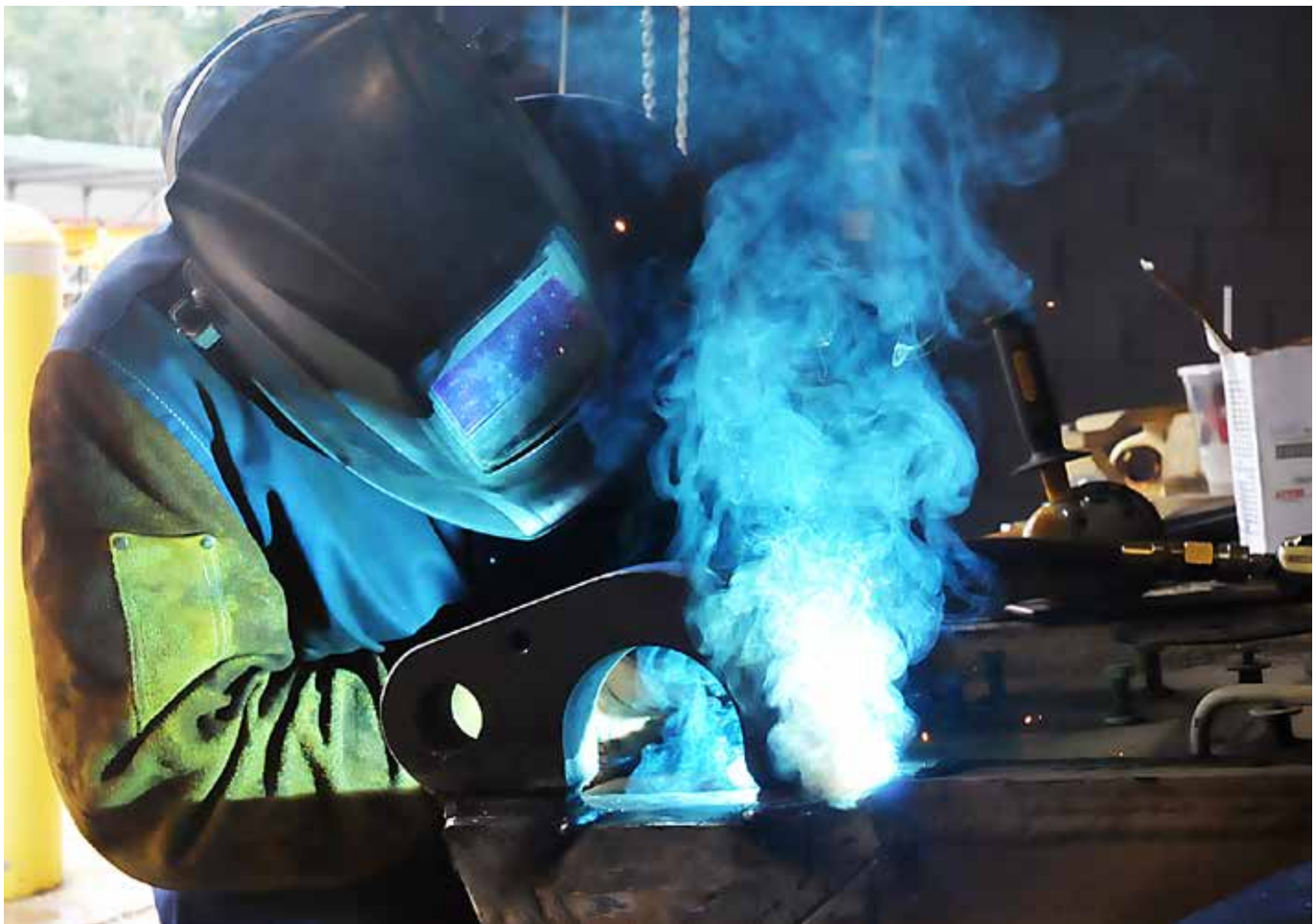
A logistics readiness center contracted employee welds the front end of an Abrams tank at Fort Benning, Ga. Vehicle maintenance is just one of the many missions of the logistics readiness centers. (Photo by Jon Micheal Connor)
