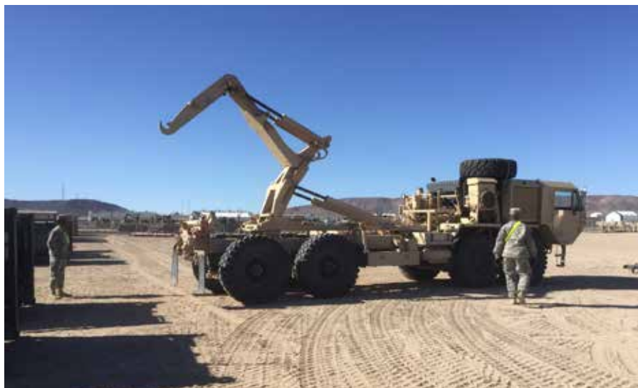
Soldiers prepare to load an M105 load handling system (LHS) compatible water tank rack onto an M1120 LHS during a 2017 National Training Center rotation at Fort Irwin, Calif.
