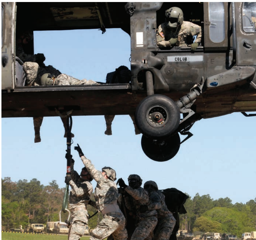
Soldiers assigned to the 24th Ordnance Company, 87th Combat Sustainment Support Battalion, 3rd Infantry Division Sustainment Brigade, attach a package to the bottom of a UH-60 Blackhawk helicopter during an exercise at Fort Stewart, Ga., on April 5, 2016. (Photo by Sgt. 1st Class Ben K. Navratil)
