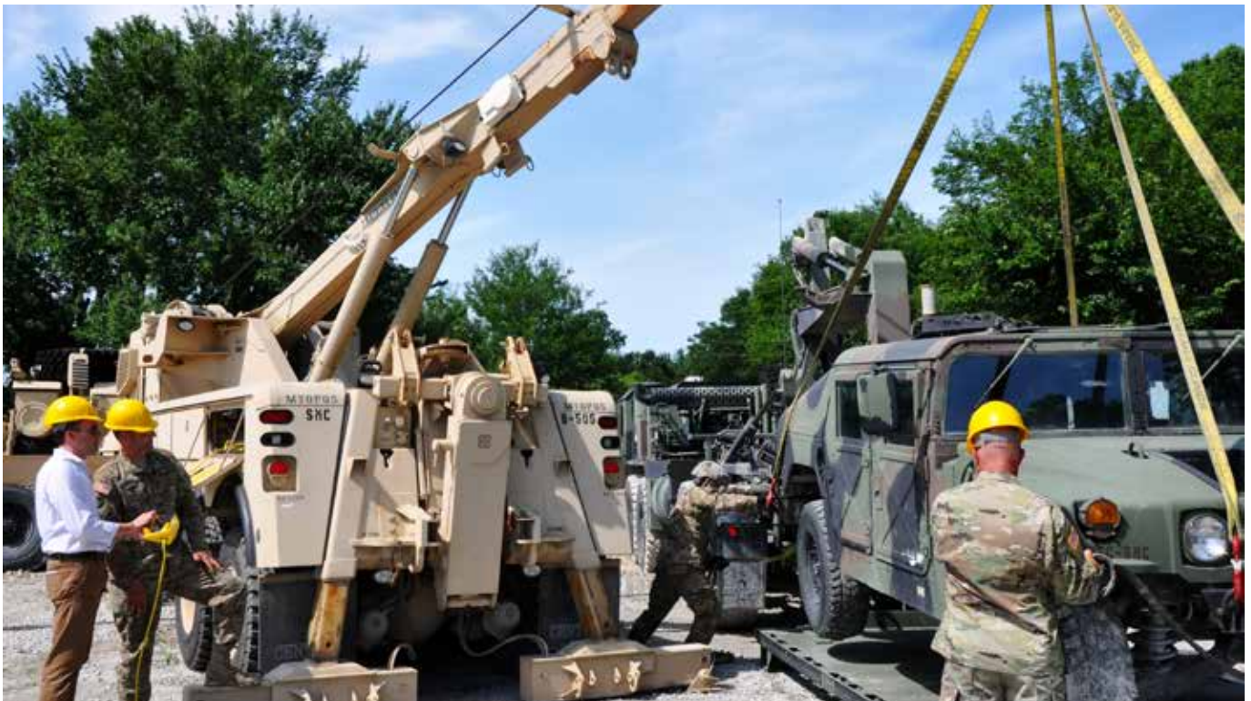
Iowa National Guard Soldiers help position a humvee onto a flatrack as then Secretary of the Army Eric Fanning maneuvers the vehicle using a mine-resistant ambush-protected wrecker. Fanning visited the Sustainment Training Center at the Camp Dodge Joint Maneuver Training Center in Johnston, Iowa, on July 14, 2016. (Photo by Master Sgt. Duff E. McFadden)
