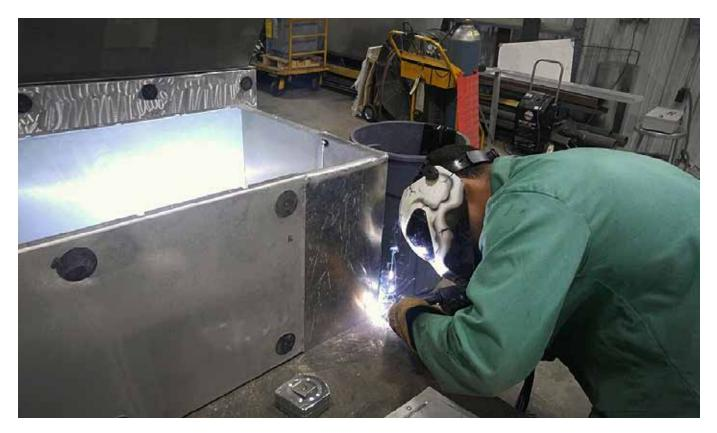
Staff Sgt. Joshua T. Lemire, an allied trades specialist with the Communications Support Detachment, Joint Communications Support Element, welds a metal fabrication. In the allied trades shop, sustainers can fabricate components for testing new communications processes and make repairs through machining and welding.
