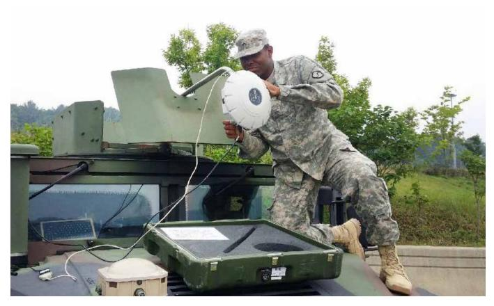
A transportation management coordinator Soldier from the 665th Movement Control Team makes adjustments to a Portable Deployment Kit interrogator installed on his crew's humvee. The interrogator is used to provide in-transit visibility of radio frequency identification tags attached to a convoy's vehicles and equipment. (Photo by 1st Lt. Carlos Moreno)
