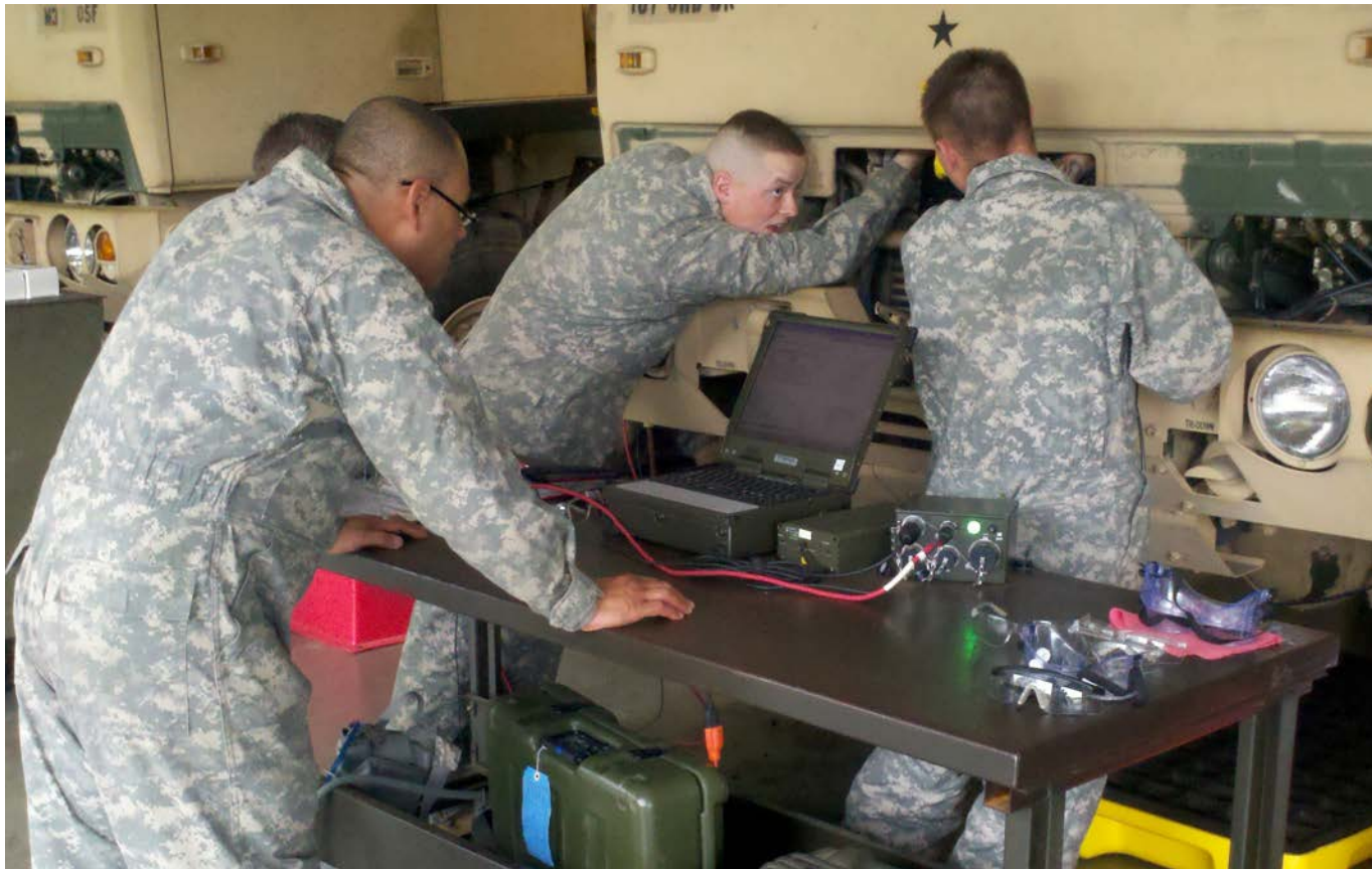
A wheeled-vehicle mechanic uses the Maintenance Support Device version 2 to diagnose vehicle faults. (Photo by Daniel R. Moody)
