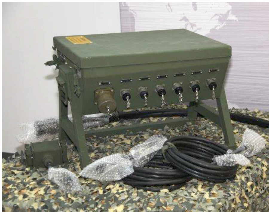
The Army's principal power distribution system, the power distribution illumination system electrical, is a rugged version of a home circuit breaker panel. It safely distributes power and is easy to connect and disconnect.
