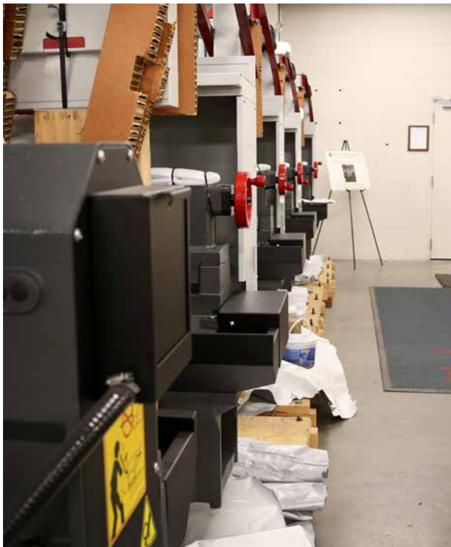
Computer numerical control toolroom lathes, like these at the Ordnance School at Fort Lee, Virginia, will be part of the metal working and machining shop set that will soon replace manual equipment sets in the field. (Photo by Julianne Cochran)
