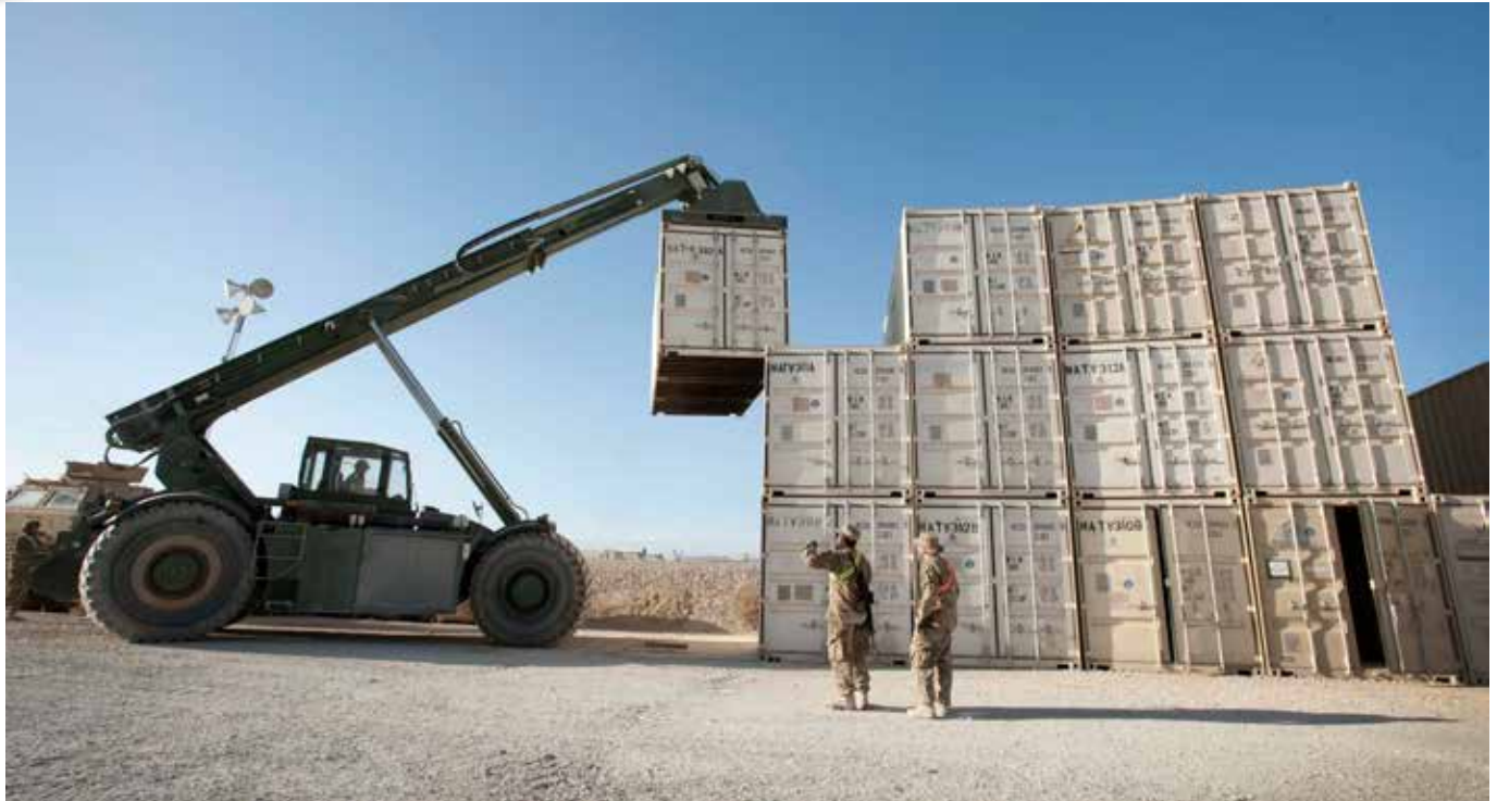
Staff Sgt. Adam Holen, 152nd Combat Sustainment Support Battalion, South Dakota Army National Guard, operates a rough-terrain container handler to move containers with guidance from two Soldiers from the Maryland Army National Guard's 1129th Transportation Company at Kandahar Airfield. (Photo by Sgt. 1st Class Theanne Tangen)
