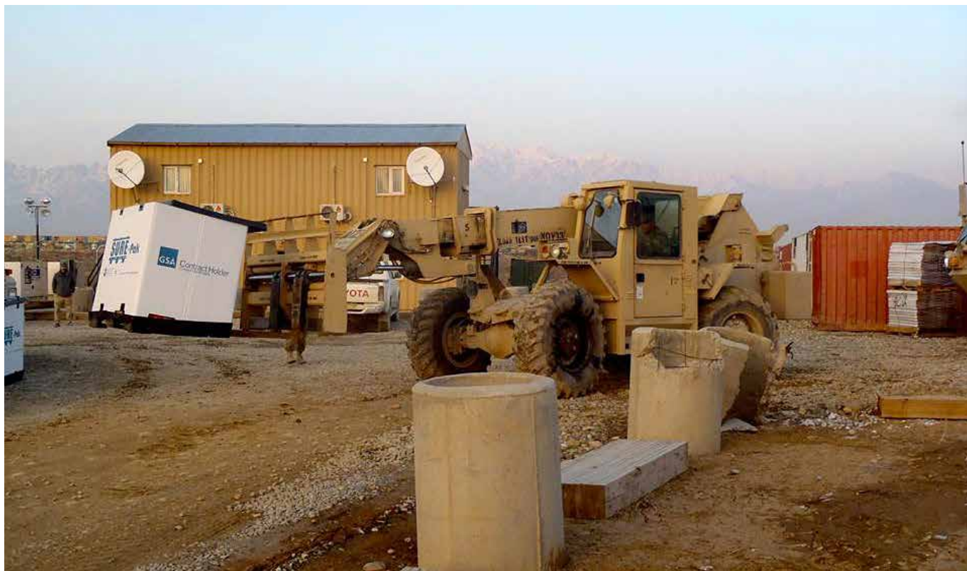
A member of a combined special operations task force logistics team operates a 10,000-pound forklift to move a “kicker box” to be uploaded onto a 5-ton medium tactical vehicle.
