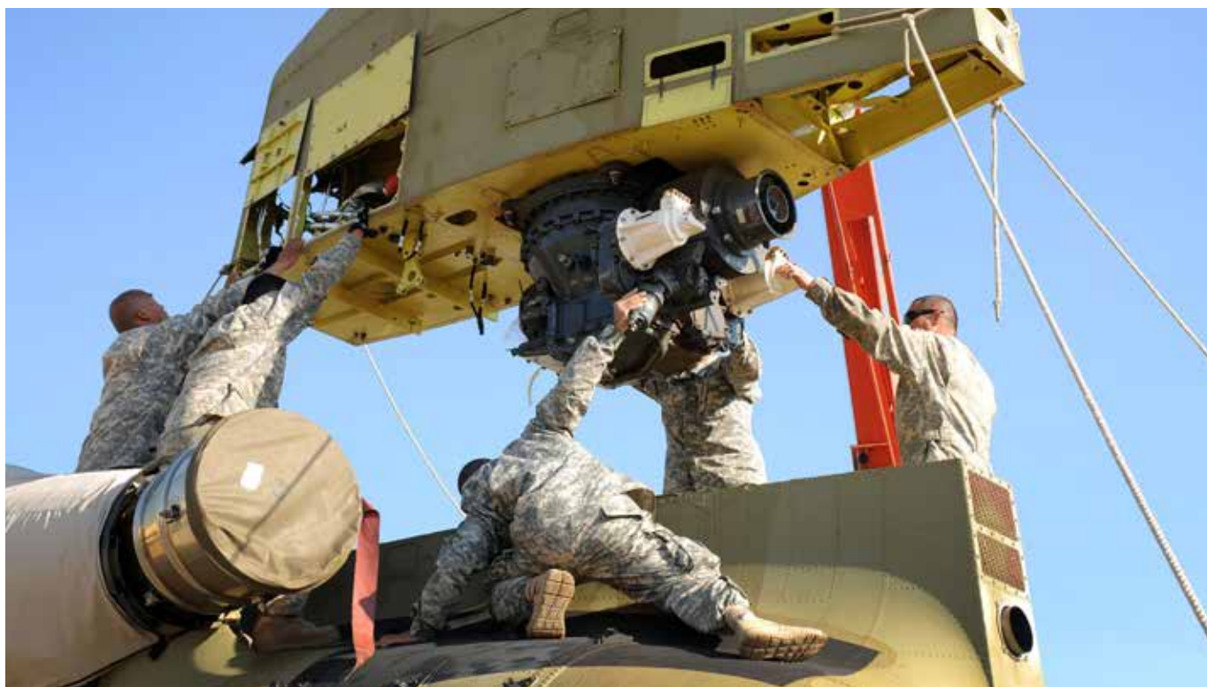
Soldiers of the Hawaii National Guard's B Company, 1-171st Aviation Regiment, place the aft transmission on one of four Chinooks that they had disassembled and transported to Botswana in support of Southern Accord 2012. (Photo by Sgt. James D. Sims)
