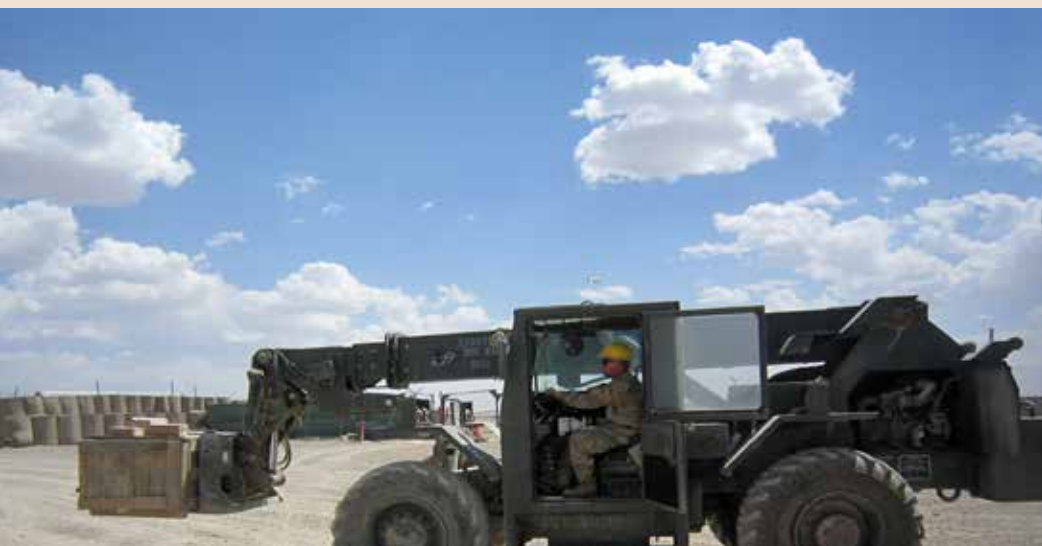
A Soldier uses a 10,000-pound variable-reach forklift to move materiel across the retrograde yard.
