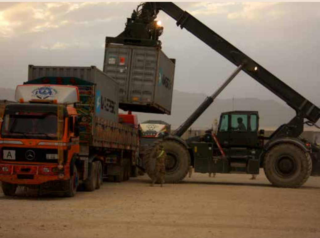
A rough-terrain container handler loads a 20-foot shipping container of retrograde materiel onto an out-bound convoy vehicle.
