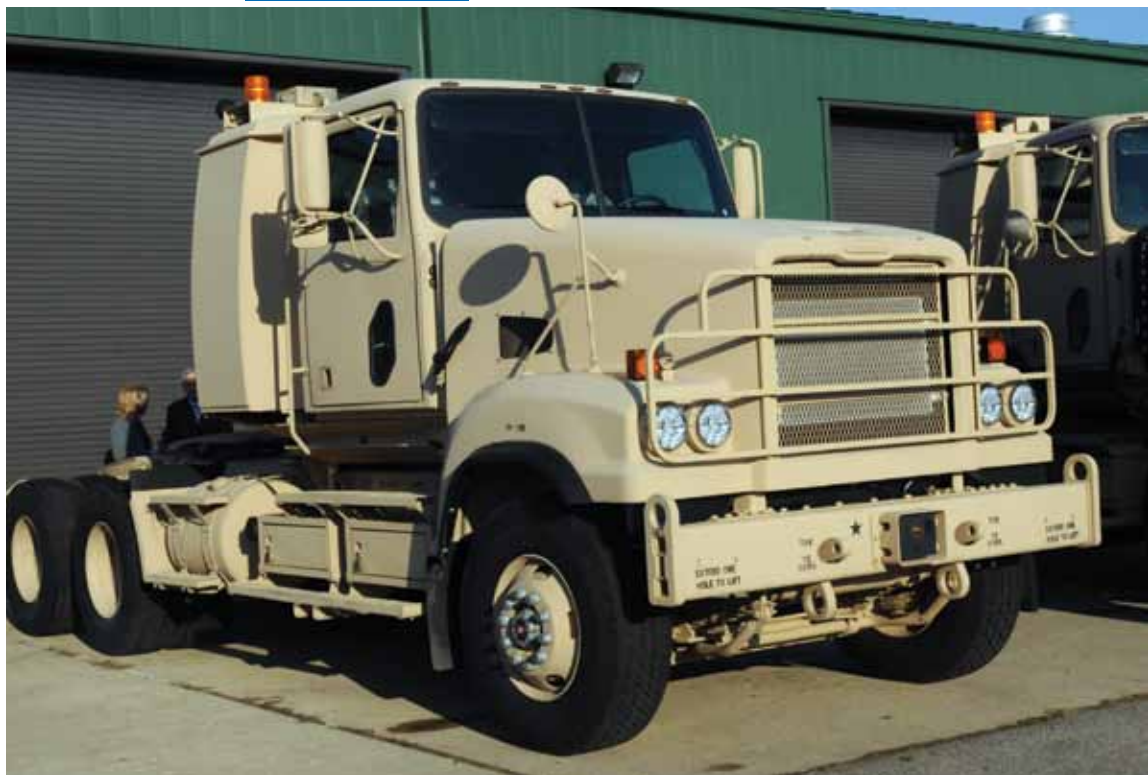
The M915A5 line-haul tractor truck is the "prime mover" in the Army's fleet of semitrailers and fuel tankers. In September, two Army Reserve units received the first 120 of 801 vehicles that the Reserve component will be issued. (Photo by MAJ Jenny Griffin, 310th Expeditionary Sustainment Command PAO)
