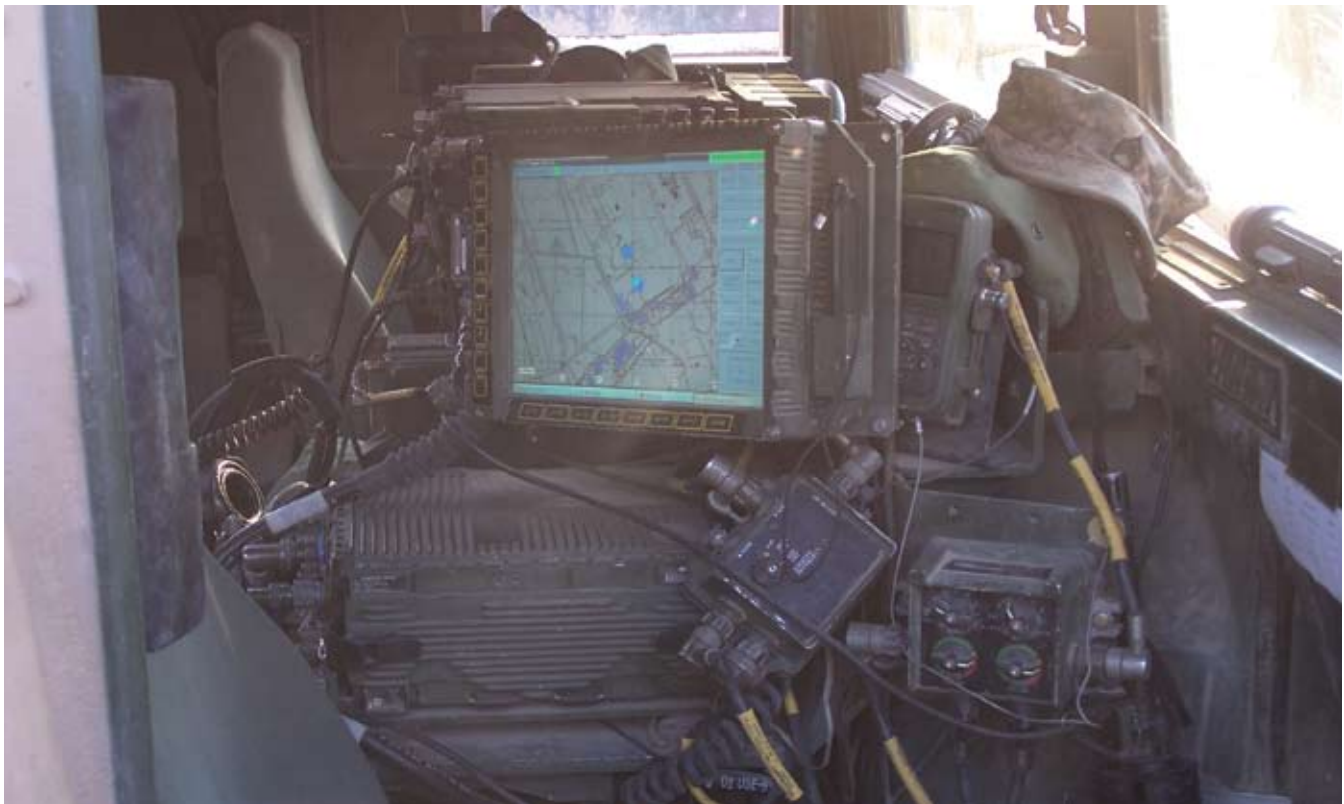
The Blue Force Tracker system gives Soldiers real-time information on troop and unit placement on the battlefield. The system allows vehicle commanders to send real-time reports back to logistics planners about conditions at the destination of a logistics convoy.
