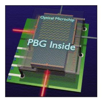
An optical microchip incorporates microphotonic devices made of PBG materials.
