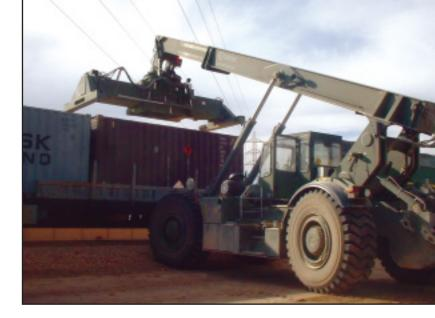
A rough-terrain container handler is used to offload containers of bottled water from railcars at AI Iskandariyah, Iraq.
