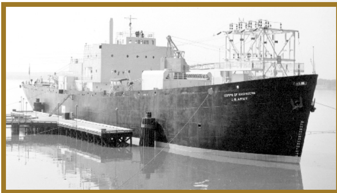
❑ The MH-1A Sturgis floating nuclear power plant, a 45-MW pressurized water reactor, was the last nuclear power plant built and operated by the Army.
