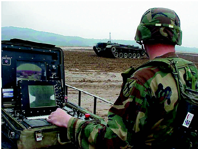
□ A soldier trains on the Panther, a remote-controlled antitank mine clearer used in noncombat environments.
