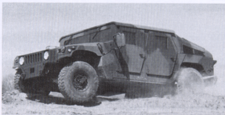
□ The M1114 up-armored HMMWV, which was fielded to troops in Bosnia in 1996 under emergency conditions, will be refurbished and retrofitted in the next 2 to 3 years.
