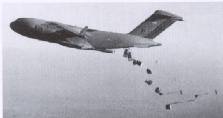
□ With an airdrop using the airdrop rails and a 7-degree nose-up angle on the aircraft, loads do not invert.
