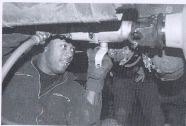
□ A mechanic installs an improved yoke in an FMTV truck.
