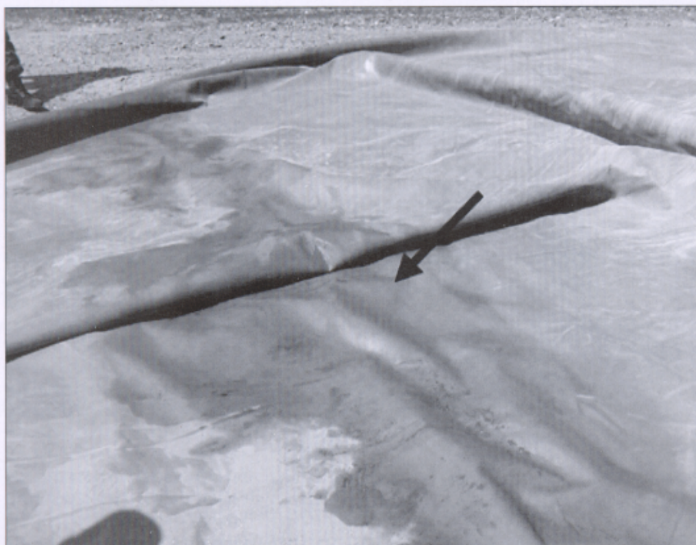
□ Arrow points to wetted surface of tank showing fuel weeping from seams during storage.
