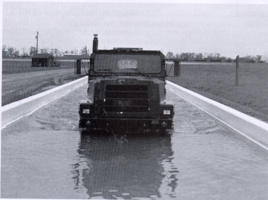
□ At the ATC, a 7-ton FMTV replacement under development for the Marine Corps is tested in a 5-percent salt solution (above) and in the grit trough (at right).
