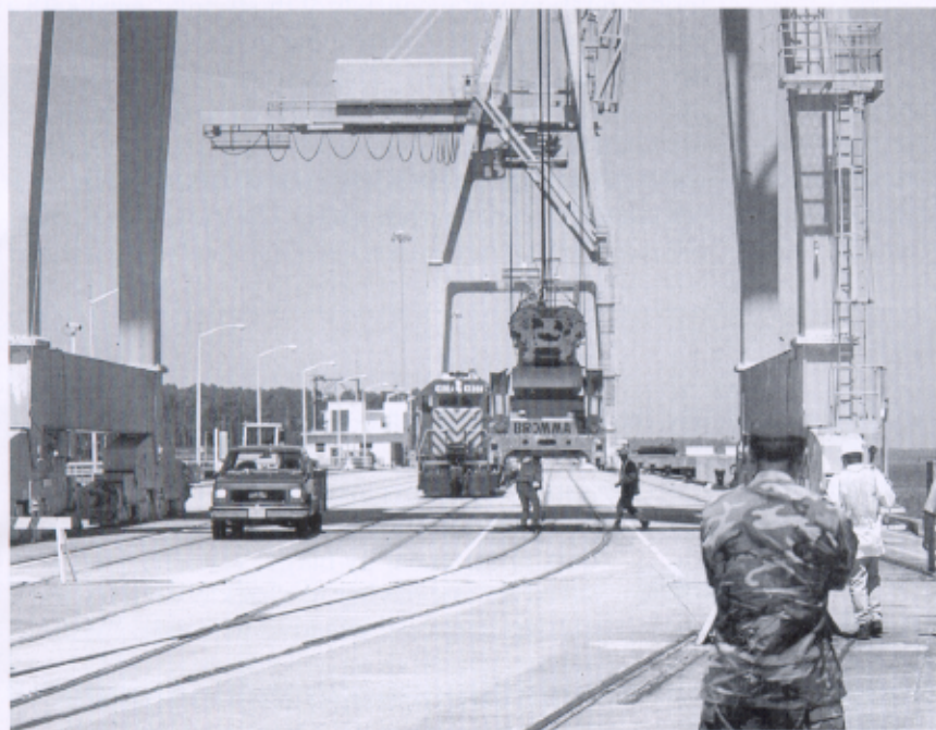
□ The DARTS spreader bar in action at Military Ocean Terminal, Sunny Point.
