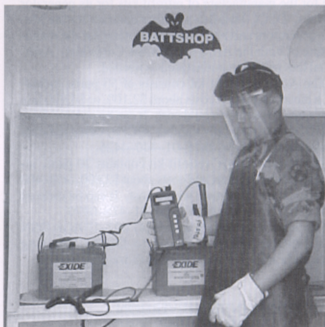
□ Batteries for use by III Corps units are tested and pulse-charged at the mobile battery shop.
