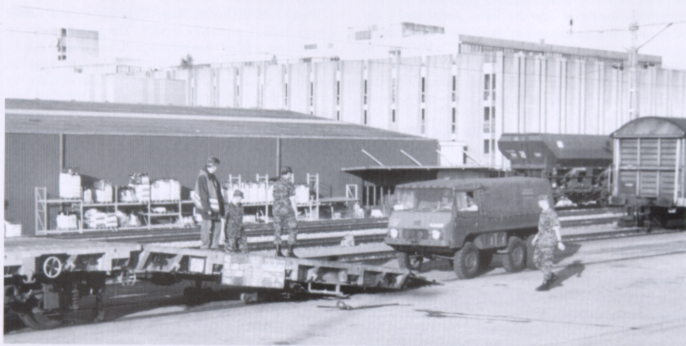
□ The last car in a train carrying Swiss equipment usually is a special car that can be converted to a mobile ramp.
