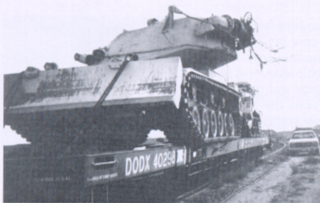
□ An M728 combat engineer vehicle turret with its boom torn off after striking a passing train.
