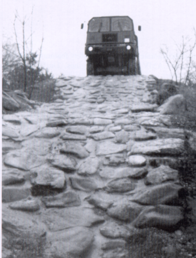
□ The surface of the obstacle course used to train Swiss truck drivers is covered alternately with rocks, gravel, sand, cobblestones, and dirt.
