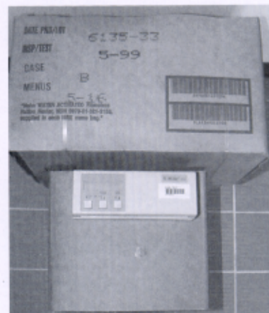
□A densitometer is used for measuring optical densities on time temperature indicators (TTI's) on MRE cases. The patch in the center of the case is a TTI.
