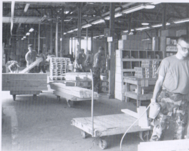
Members of the 125th Transportation Company (Cargo Transfer), USAR, helped employees at Blue Grass Army Depot make blocking and bracing materials for munitions shipments.
