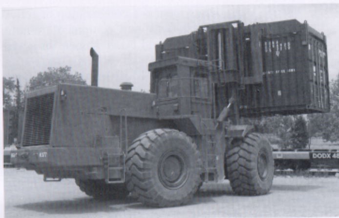
□The rough-terrain container handler lifts a MILVAN loaded with 750-pound bombs onto a railcar at Blue Grass Army Depot.
