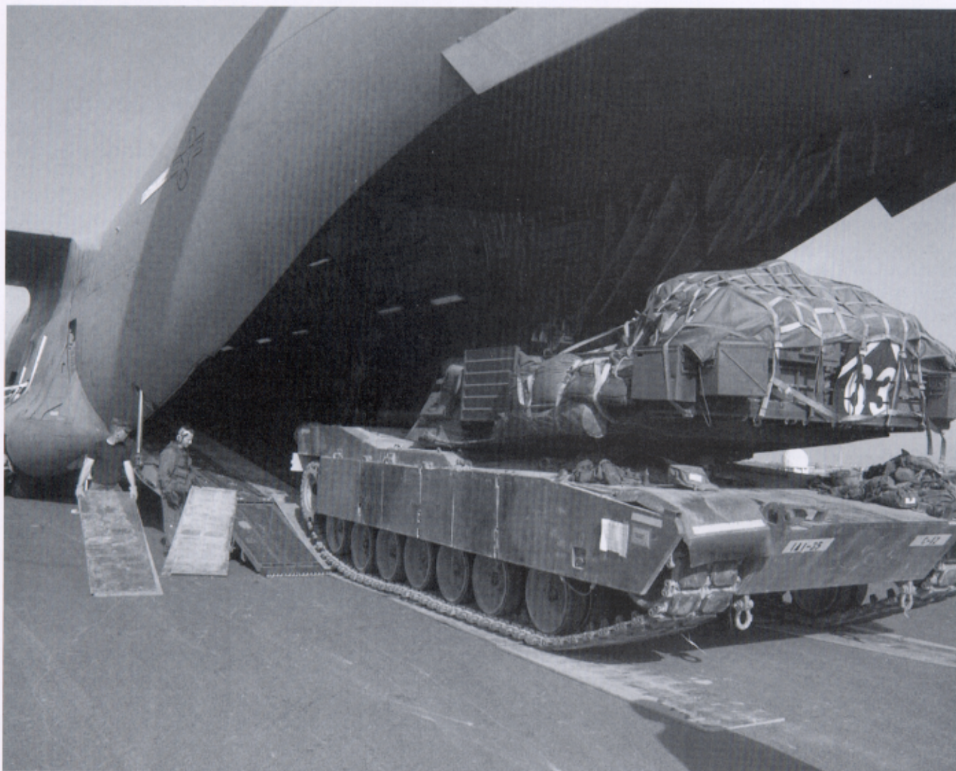
□ Soldiers and airmen guide an M1A1 Abrams main battle tank onto a C-17A Globemaster III for transport.
