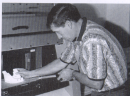
□ Rock Island Arsenal's 3D printer produces models that are detailed to a resolution of .013 inch.
