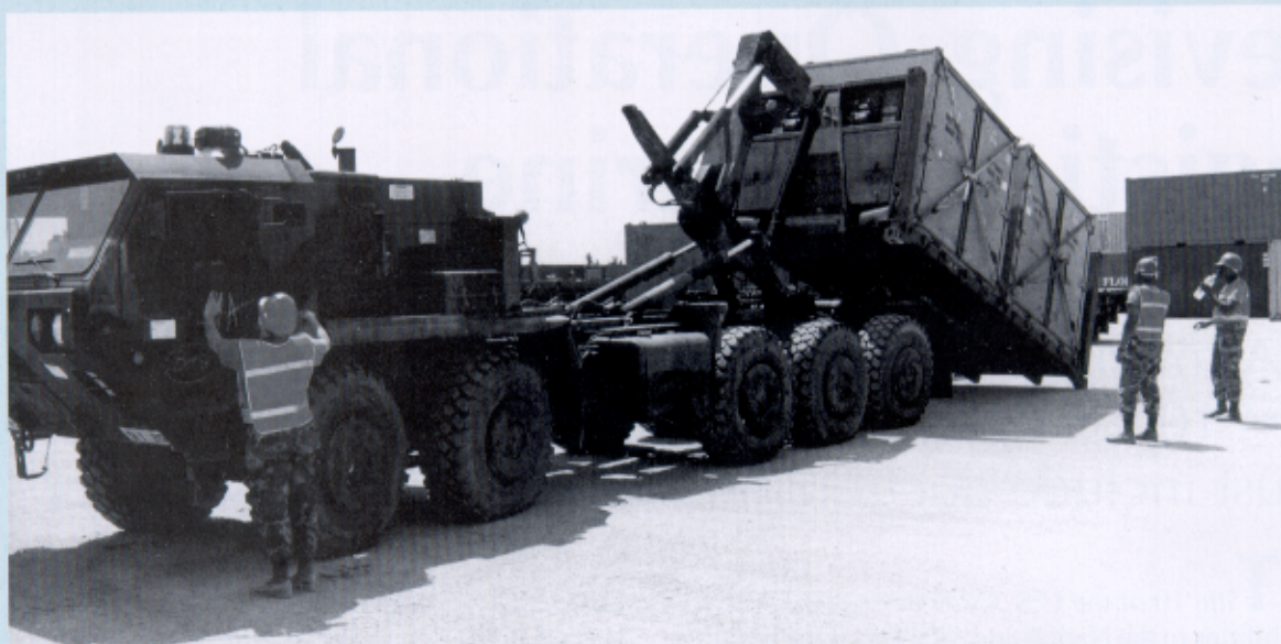
□ Using a palletized loading system, soldiers at the Thessaloniki docks place a container on a truck. The container holds a standard deployment package.
