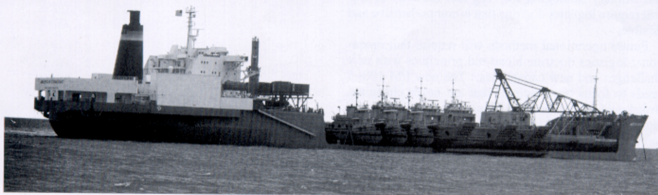
□ The American Cormorant sits off the coast of southern England, ready to partially submerge so it can offload the vessels on board. The ship is the only semisubmersible cargo vessel in the Army Pre-positioned Stocks system.
