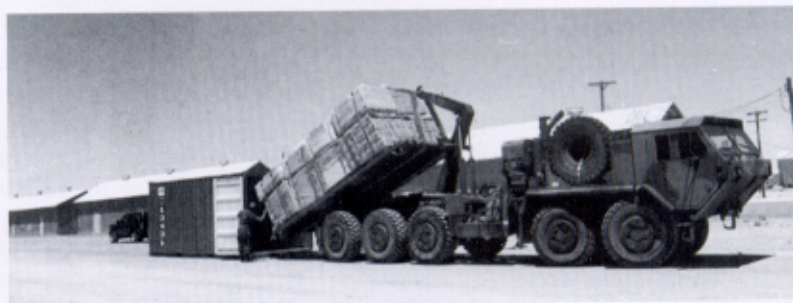
□ A container roll-on-roll-off platform removes a STRATPAK from a van for transfer to a flatbed truck.
