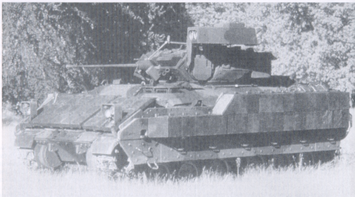
□ The Bradley fighting vehicle is one of the Army's reliability success stories. Testing of the A2 version has achieved 750 mean miles of operation between failures.
