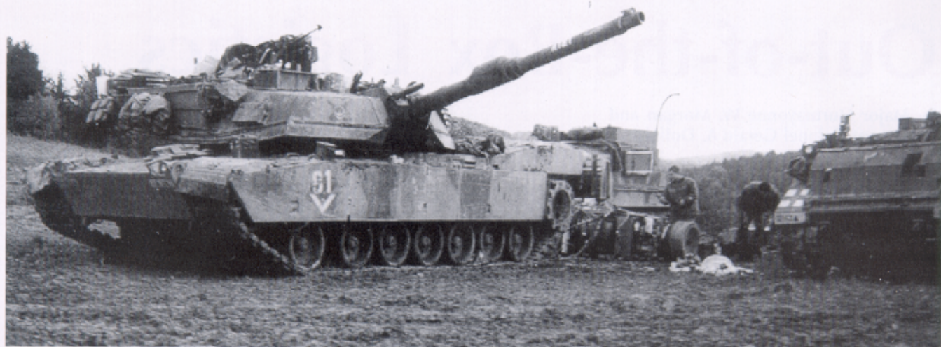
□ Soldiers of the 51st Maintenance Battalion repair an M1 Abrams tank at a unit maintenance collection point.
