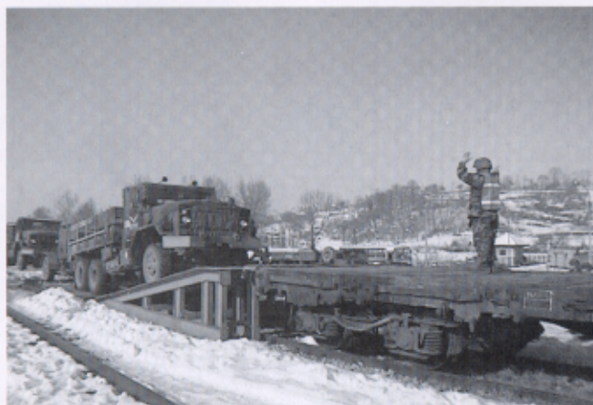
□ Above, a truck commander guides a driver onto a flatcar—the most dangerous part of the retrograde operation. At right, excess equipment sits on a railcar headed for the Central Region in Germany.
