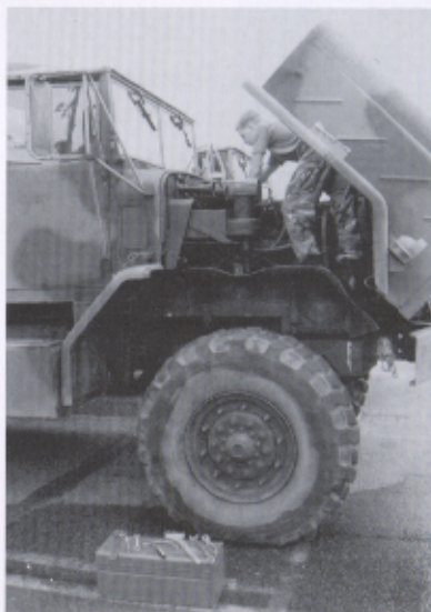
□ Second-echelon maintenance of tactical vehicles, such as this 5-ton cargo truck, is performed by mechanics who deploy with the rifle company.
