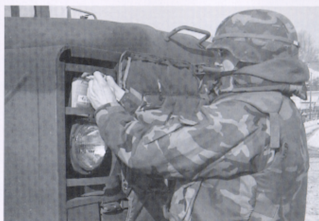
□ Rolling stock is washed at the Lukavac washrack before it is staged for loading onto a railcar. At right, a soldier attaches a radio frequency tag to a vehicle being shipped to the Central Region.
