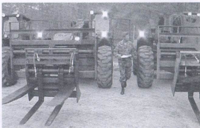
□ A 528th Special Operations Support Battalion soldier conducts preventive maintenance checks and services on the ATLAS.
