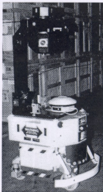
□ As it patrols a warehouse at Anniston Army Depot, the MDARS robot reads RF tags that are affixed to items in storage.
