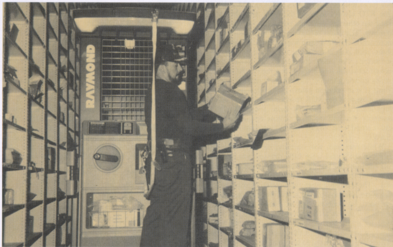
One of the two types of materials-handling vehicles obtained for the modernized warehouse, the stock selector truck moves between bins and lifts the operator to the bin level he wants.
