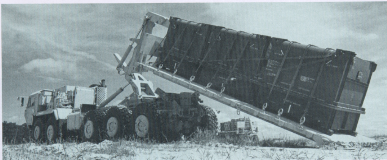
□ A self-contained, hydraulic load-handling system in the body of the truck loads and unloads the flat-racks from both the truck and trailer.
