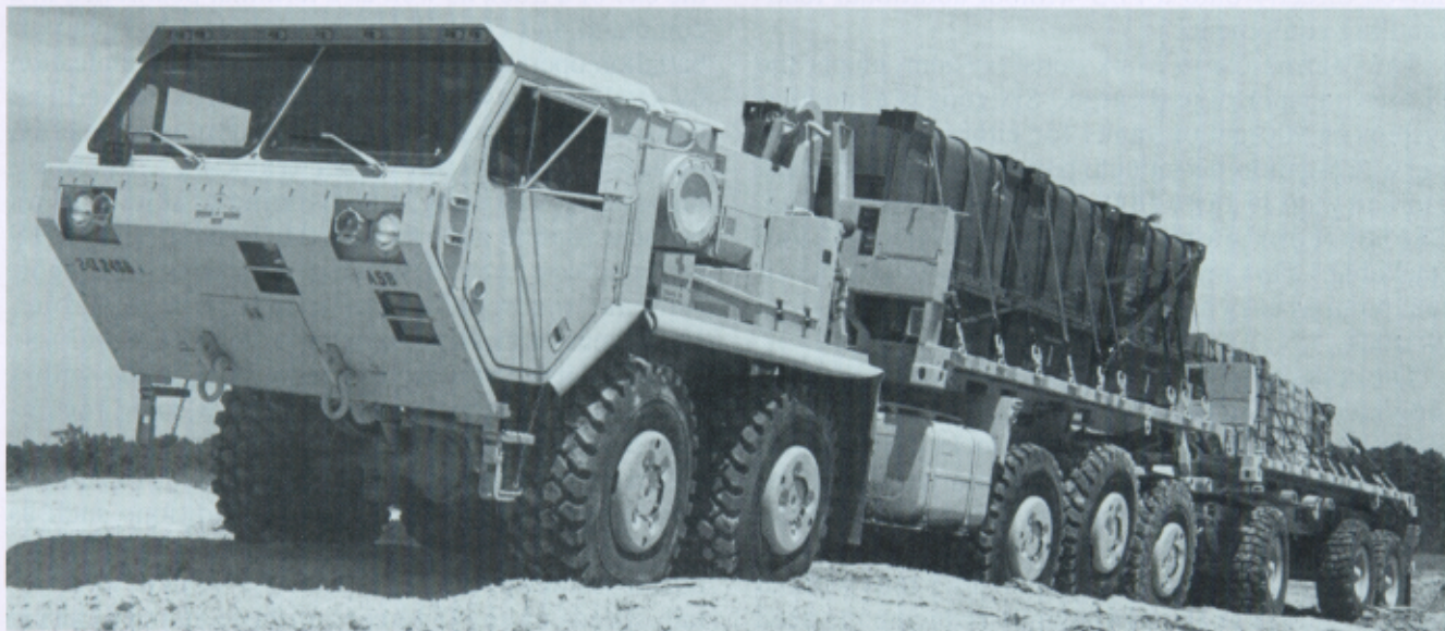
□ The PLS consists of a truck, a trailer, and two demountable cargo beds, or "flatracks."
