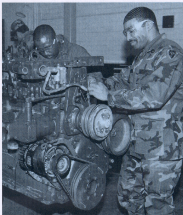
□ Two soldiers from the 732d Maintenance Company (GS), North Carolina ARNG, complete final assembly of a Cummins NHC 250 engine. The engine was rebuilt by their company during annual training at the GS Equipment Maintenance Center-CONUS (EMC-C), part of the National Maintenance Training Center at Camp Dodge, Iowa.
