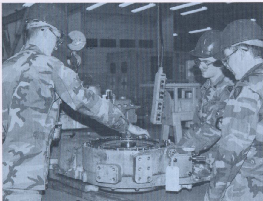
□ Soldiers from the 732d Maintenance Company (GS), NCARNG, reassemble a rebuilt Allison X1100-3B M1 tank transmission output housing. M1 Abrams tanks are among the force modernization equipment on which maintenance companies train at the EMC-C.
