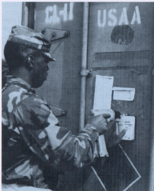
□ A soldier of the 7th Transportation Group attaches a Savi 128-kilobyte radio frequency tag to a prepo container.
