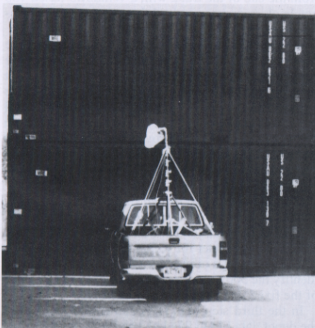
□ A fixed interrogator mounted on a pickup truck is used to burn data on radio frequency tags attached to containers.
