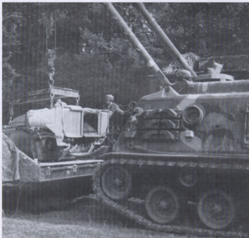
□ This soldier (left) is checking an engine for malfunctions before it is reinstalled in an M1A1 tank. A repaired FUPP (above) is being loaded for movement back to the front line.
