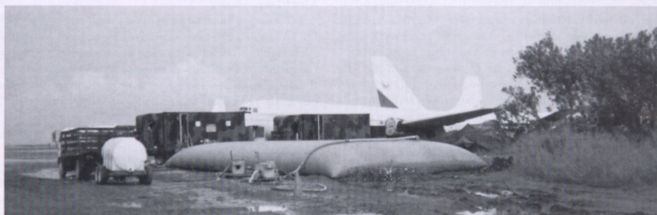
□ A 3,000-gallon-per-hour reverse-osmosis water purification unit at Port-au-Prince International Airport provides fresh water for the joint task force.
