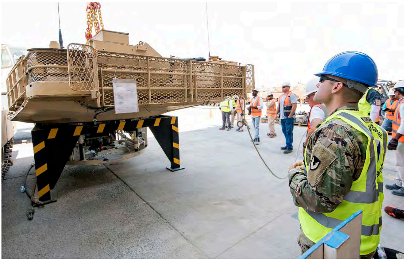
Sgt. 1st Class Robert Ford, quality assurance for tanks, 401st Army Field Support Battalion-Kuwait, watches as contractors at Army Prepositioned Stocks-5 work to lift a 30-ton turret, Camp Arifjan, Kuwait, Sept. 23. (Photo by Kevin Fleming)
