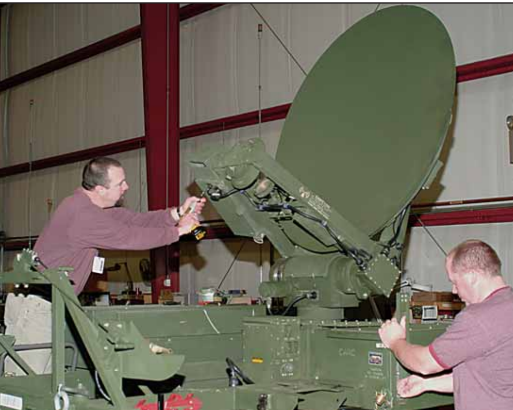
Technicians repair an AN/TSC-154 Secure Mobile Anti-jam Reliable Tactical Terminal (SMART-T) at Tobyhanna Army Depot, Pennsylvania. The SMART-T is a Military Strategic and Tactical Relay (MILSTAR) satellite-compatible ground communications terminal that provides worldwide data and voice communications from a stationary mission site. This repair is part of a SMART-T reset program. Tobyhanna technicians have repaired 19 SMART-T systems for the Army and will repair 13 for the Marine Corps. (Army photo by Steve Grzedzinski)
